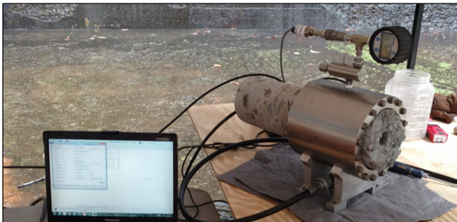
Figure 10. Biaxial test chamber used to determine elastic modulus.
